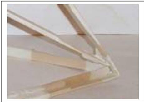
Using a couple of pieces of tape connect the other end of the catapult arm to the place where the three triangles meet. (Note: the catapult arm should go through the inside of the triangles) This is a bit tricky to do but do your best and try to secure the catapult arm firmly. But it has to move freely. Think of the tape as being a kind of a hinge.
